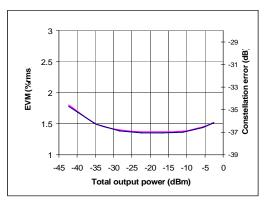
Figure 13. EVM function of gain control
