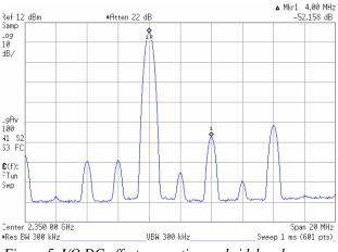
*Figure 5. I/Q DC offset correction and sideband nulling.*
