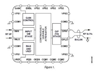
Figure 9. ADL5330 1 MHz to 3 GHz 60 dB Linear-indB VGA.
