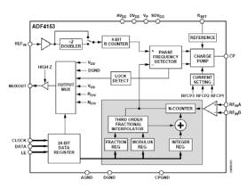
Figure 7. ADF4153 4 GHz Fractional-N Synthesizer.
