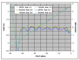
Figure 14. AD8362 RMS Detector Output Voltage and linearity error vs. System Output Power and Signal Type
