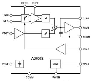
Figure 10. AD8362 50 Hz to 2.7 GHz 60 dB  $TruPwr^{TM}$ Detector
