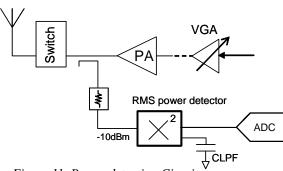
Figure 11. Power detection Circuit
