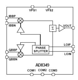
*Figure 4. AD8349 700 MHz to 2700 MHz Quadrature Modulator*
