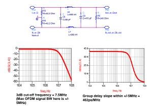
Figure 3. Baseband Bessel Low Pass Filter
